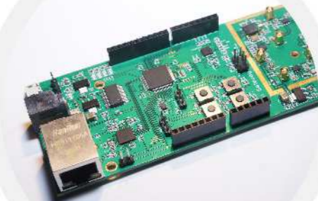
TIPoT long range communication board and Ethernet gateway
